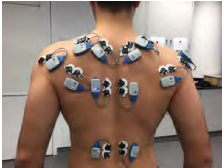
Figure 2.2 Example of placement of EMG sensors on the back muscles
