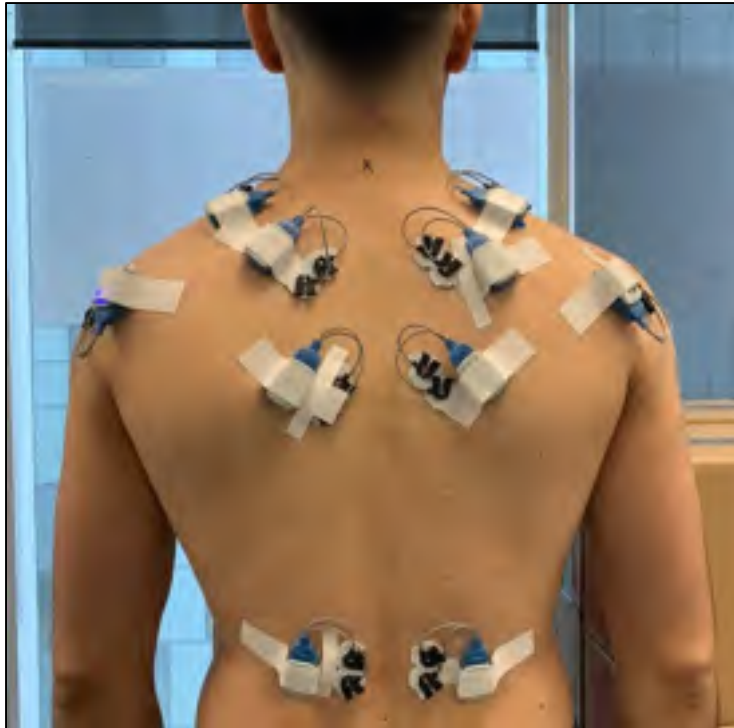
Figure 2.3 Pasting measuring tape over the electrodes and EMG sensors.
