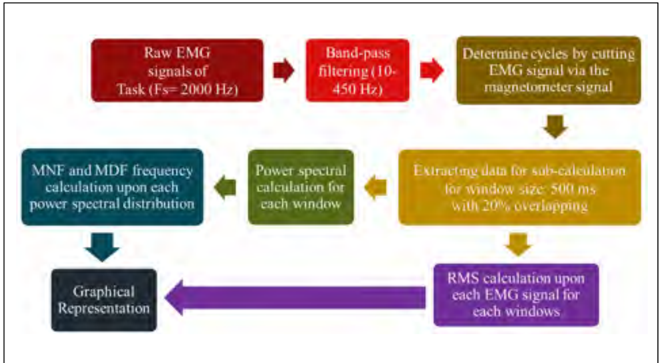
Figure 2.5 Procedure of MDF & MNF calculations
