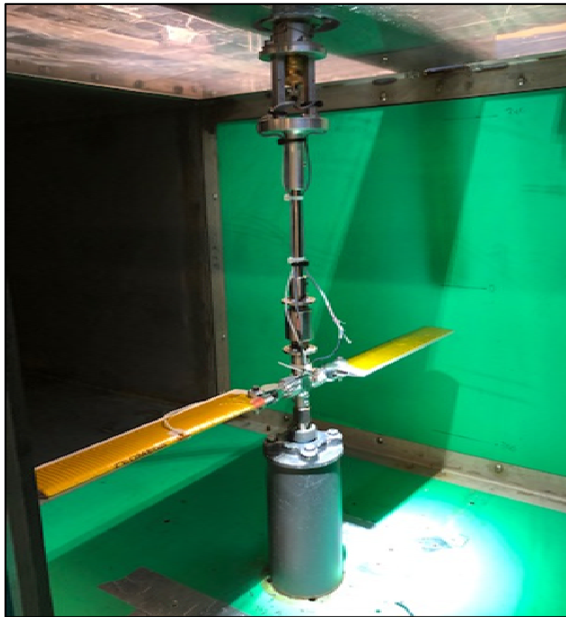
Figure 3.8 Rotor Prototype in Wind Tunnel with Exposed Heating Elements
