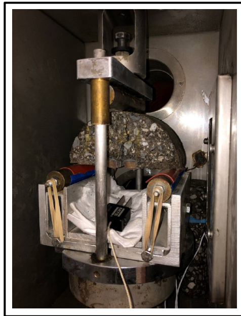
Figure 4. 4 SCB test fixture
