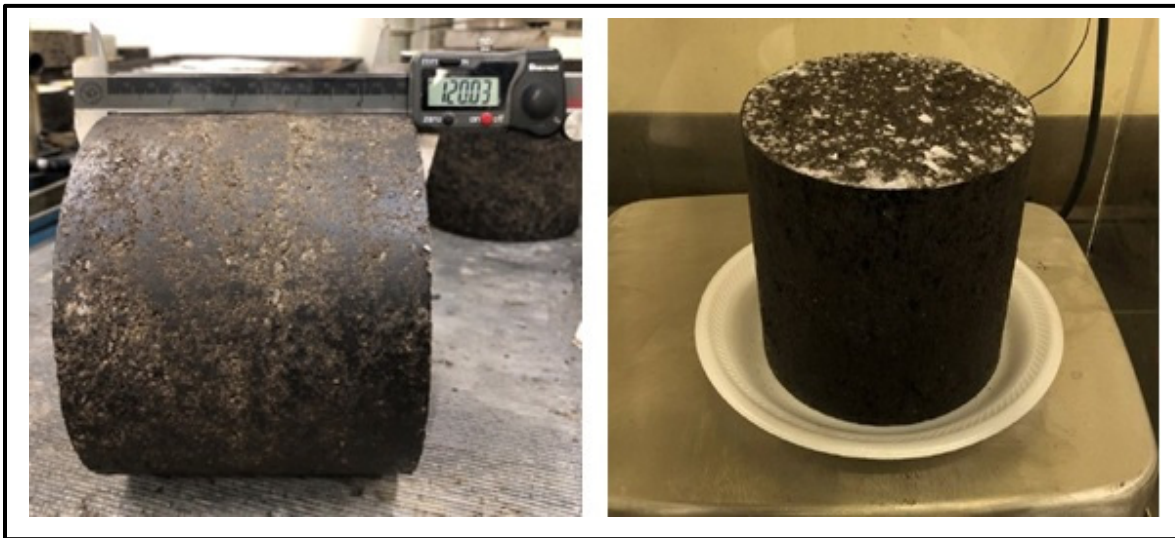
Figure 4. 2 Compacted specimens with SGC
