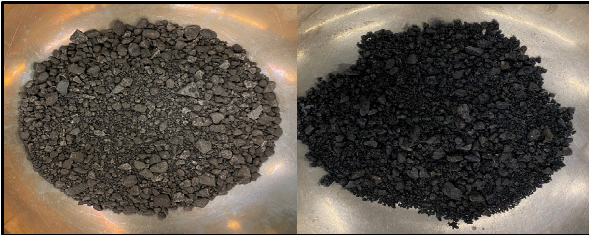
Figure 4.5 RAP (left) and rejuvenated whole-RAP loose mixture prepared at 100 °C (right)
