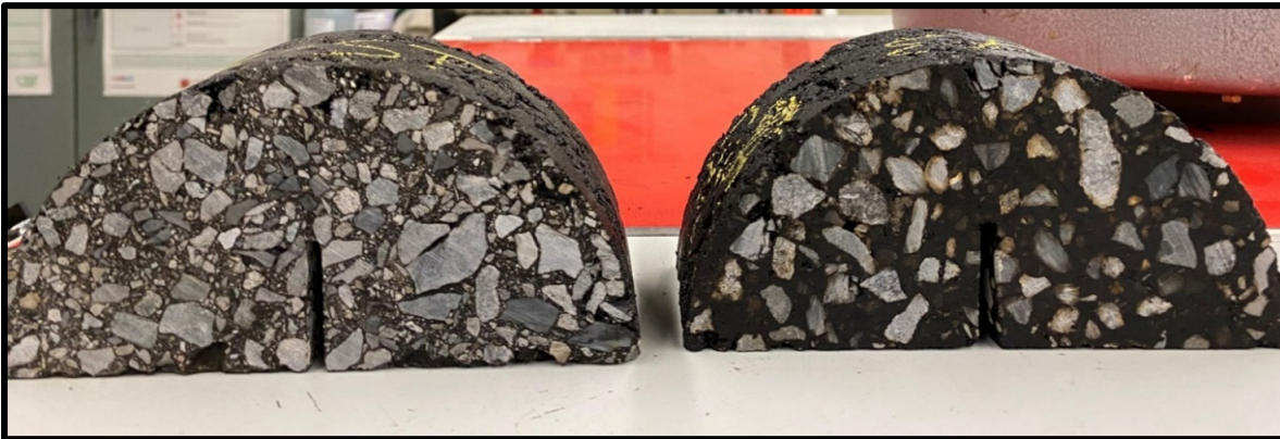
Figure 4.10 SCB sample before (left) and after (right) LT aging
