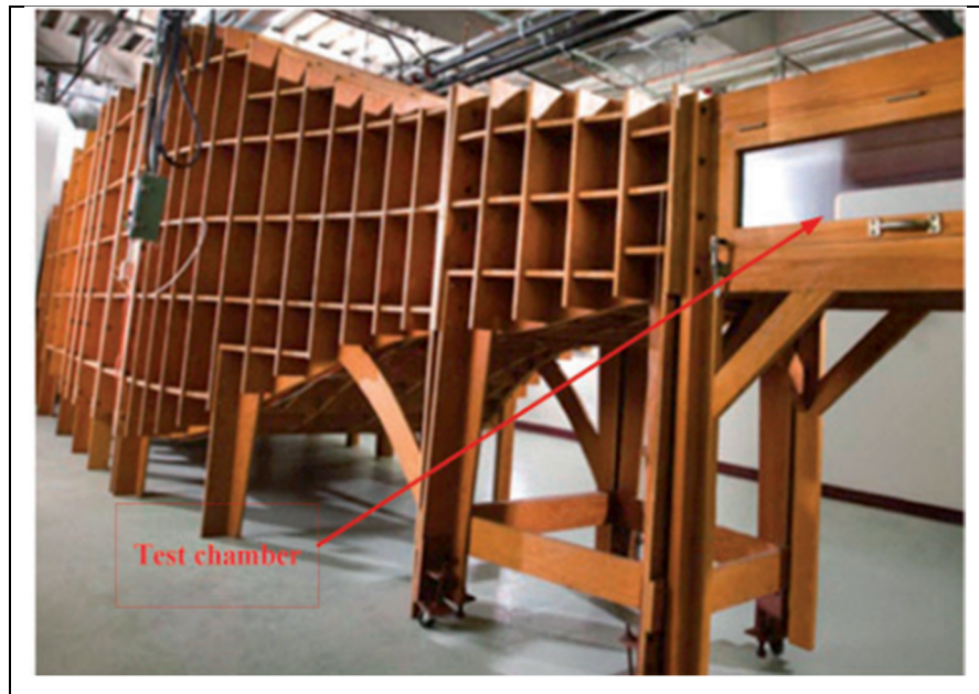
Figure 6.1 LARCASE Price-Paidoussis subsonic blow down wind tunnel
