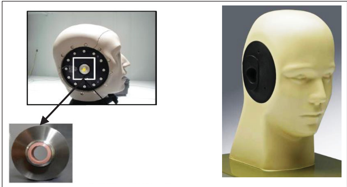
Figure 1.3 Left, G.R.A.S 45CB without the circumaural flesh simulation and the cylindrical ear canal with flesh simulation
