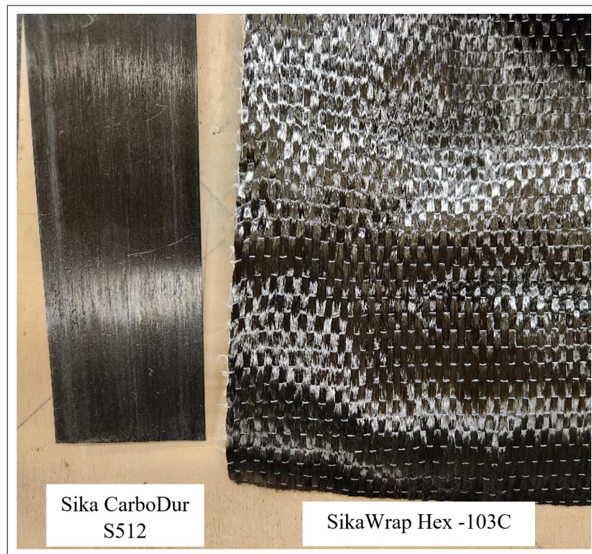
Figure 1.14 CFRP composites used in the experimental program
