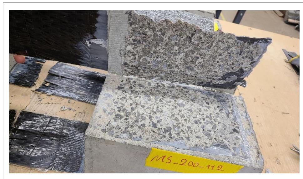
Figure 2.4 Concrete cover failure mode
