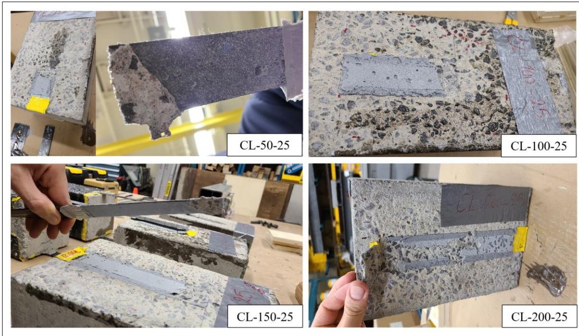
Figure 5.4 Failure modes of specimens with CFRP laminate during cyclic loading
