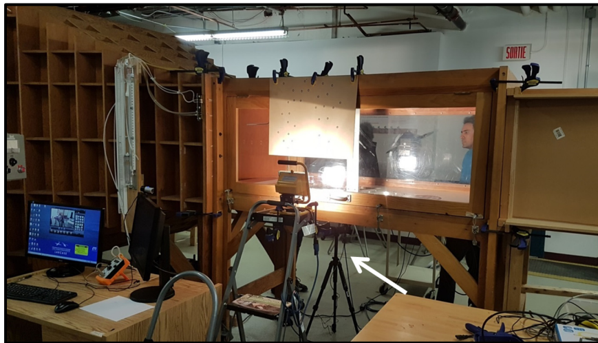
Figure-B II-3.2 Video recording installation and wind tunnel setup. The camera position is shown by the white arrow
