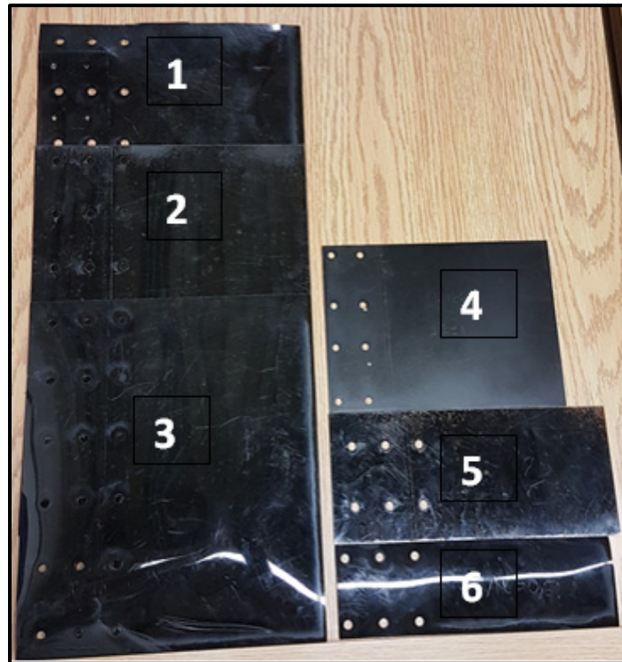
Figure-B II-2 Foils tested for this thesis. Aspect ratios are: 1)AR=4, 2)AR=3, 3)AR=2, 4)AR=1, 5)AR=0.75, 6)AR=0.5
