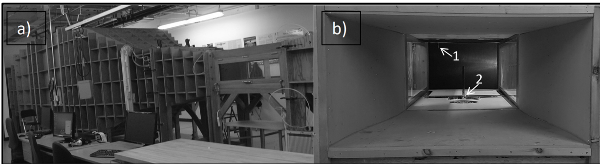
Figure 4. 1 a) The Price–Païdoussis Open Return Subsonic Wind Tunnel. b) Pitot tube location (1) and aerodynamic scale location (2)
