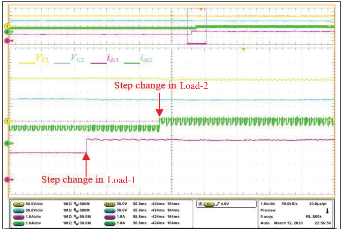
Figure 4.10 Experimental results for the DC voltages and currents during the load variations
