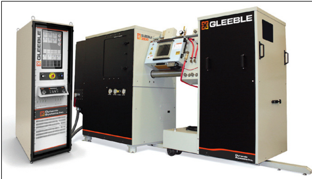
Figure 2.6 Thermo-mechanical simulator Gleeble 3800 Taken from Dynamic Systems (2023)
