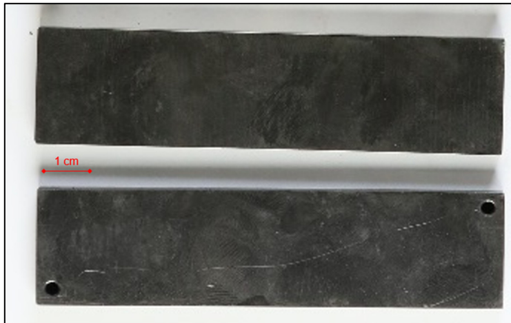
Figure 2.13 Size of 4340 coupons used for set 4
