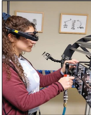
Figure A.II.1 Assembly of brackets on a simulated plane engine using smart glasses
