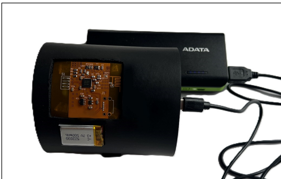
Figure 4.1 Casing design for the flexible WWD
