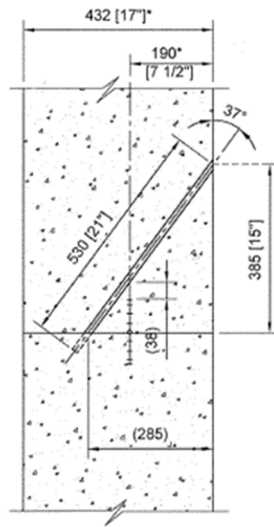
Figure 3.3 Drilling parameters for P11
