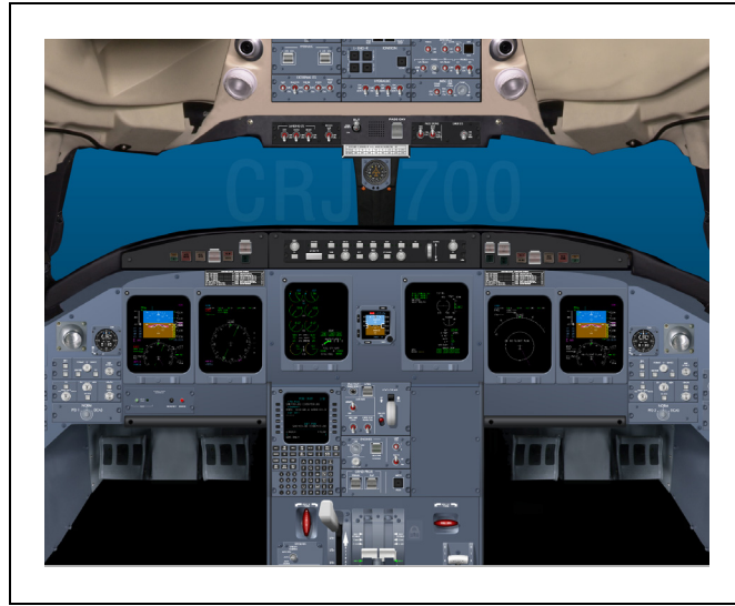
Figure 4.1 Bombardier CRJ-700 Virtual Research Equipment Simulator (VRESIM) used for the validation of the proposed methodology
