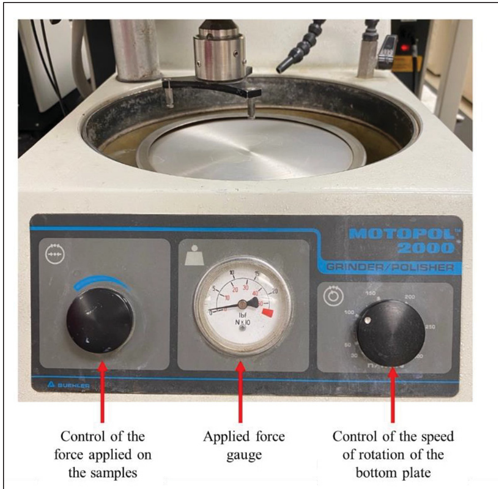
Figure-A III.3 Bottom control panel, where the force applied on the samples during polishing and the speed of rotation of the bottom plate can be tuned
