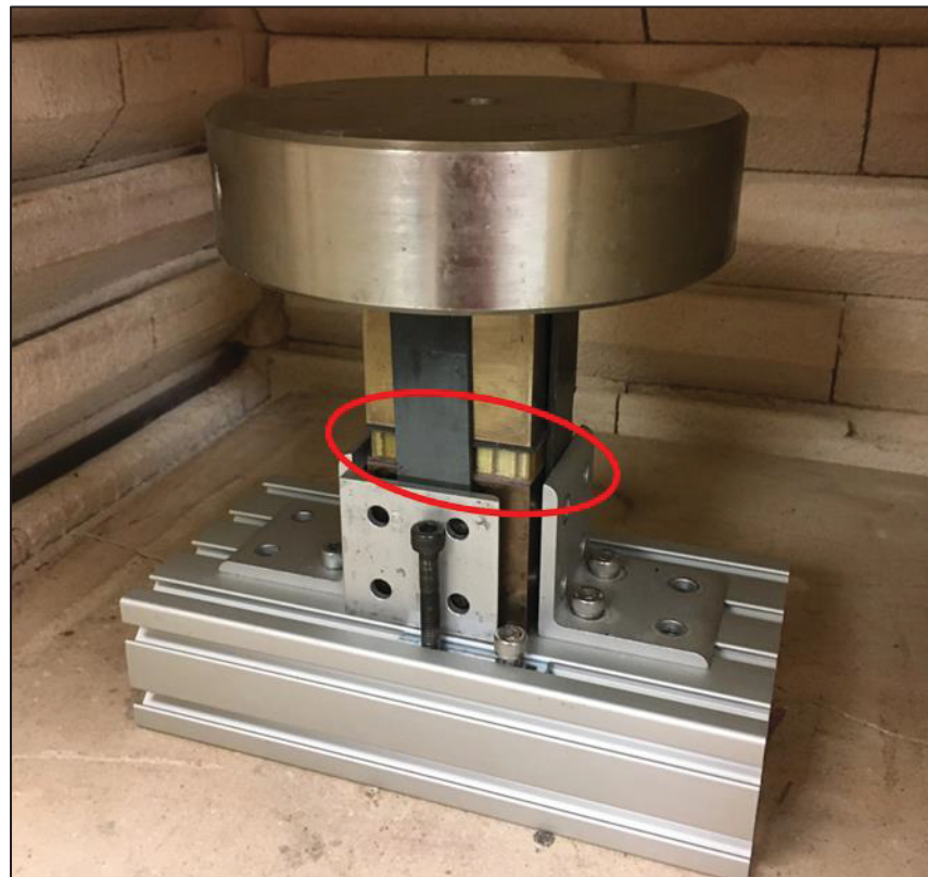
Figure-A IV.2 Alignment setup in the oven. The red circle highlights the position of the sandwich sample. The weight placed on top is used to apply pressure during curing
