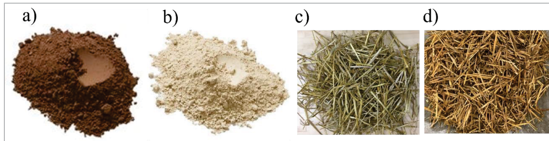
Figure 3.1 Photographic images of a) the red clay, b) the beige clay, c) the dry fibres, and d) the wet fibres
