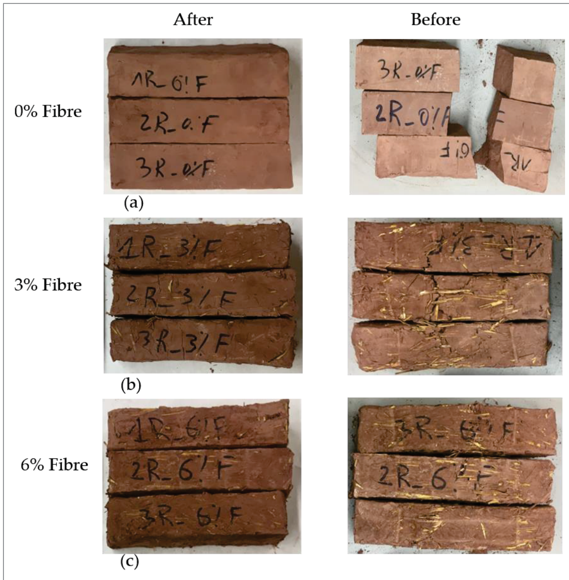
Figure AC-2 Condition of the samples after and before flexural testing
