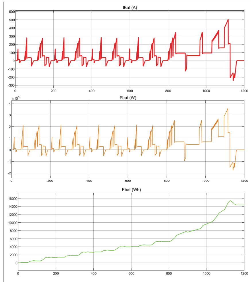
Figure 4.8 Correlation between battery power and current, validating the battery's consistent or ascending energy levels in accordance with the non-plug-in hybrid vehicle design
