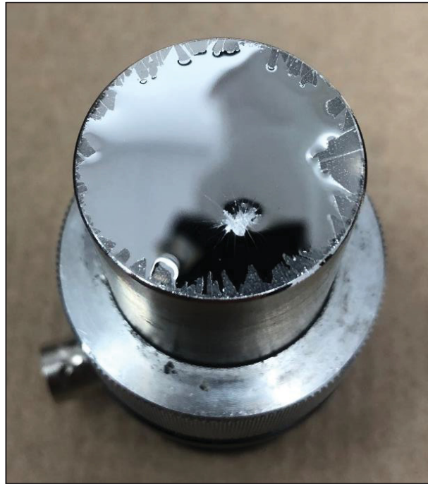
Figure 2.8 Adhesion of the smooth oxide layer on Titanium matching layer, the film is distributed over almost the entire surface
