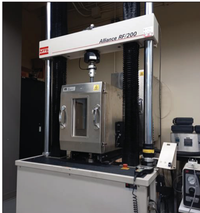
Figure A II-2 – Assembly of the environmental chamber coupled to the Alliance RF/200 MTS universal testing machine used for the ambience of the tensile tests at -40^{\circ}\text{C}
