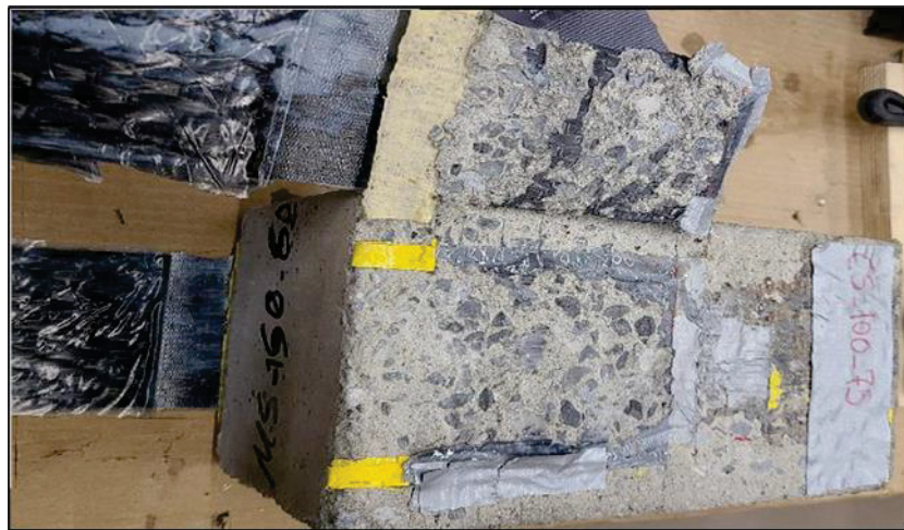
Figure 1.9 Concrete substrate failure of Concrete/CFRP joint Taken from (Fathi, El-Saikaly et al., 2023, p. 6)
