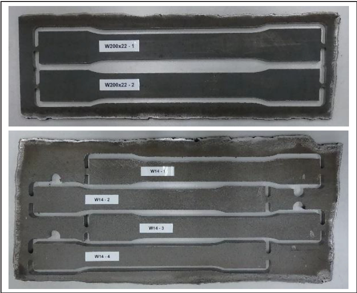
Figure 4.2 Steel coupons extracted from the beams
