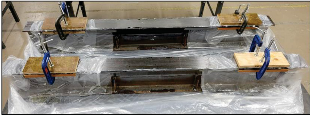
Figure 4.4 Curing of the SikaWrap fabric
