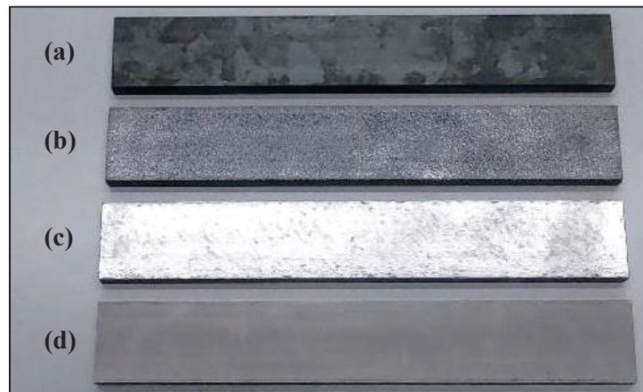
Figure 3.1 Steel plate surface; (a) Before surface treatment; (b) After applying needle scaler; (c) After applying sandpaper machine; (d) After sandblasting
