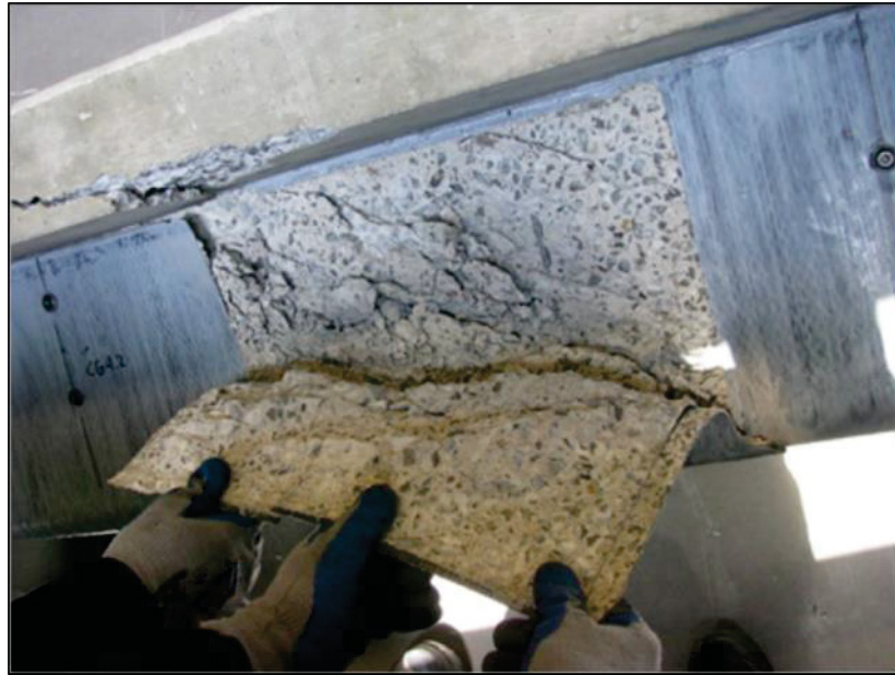
Figure 1.8 Debonding failure in RC beam retrofitted with FRP Taken from El-Saikaly and Chaallal (2015, p. 7)
