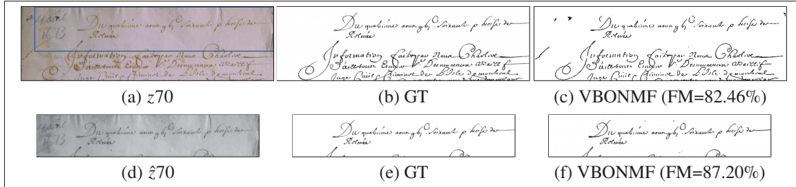
Figure 5.9 VBONMF text extraction results on the sample z_{70} from the MSTEx-1 dataset and the sample \hat{z}_{70} from the HISTODOC1 dataset. The blue box in (a) shows from where the image in (d) was cropped, approximately. (b) and (e) are the corresponding GT for (a) and (d), respectively, (c) and (f) are the final binary images
