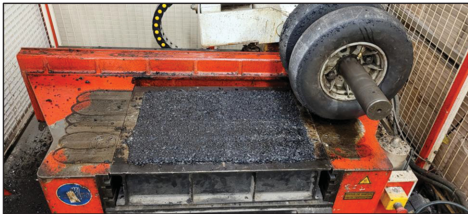
Figure 3.19 Photo d'une plaque 500 mm x 180 mm x 150 mm
