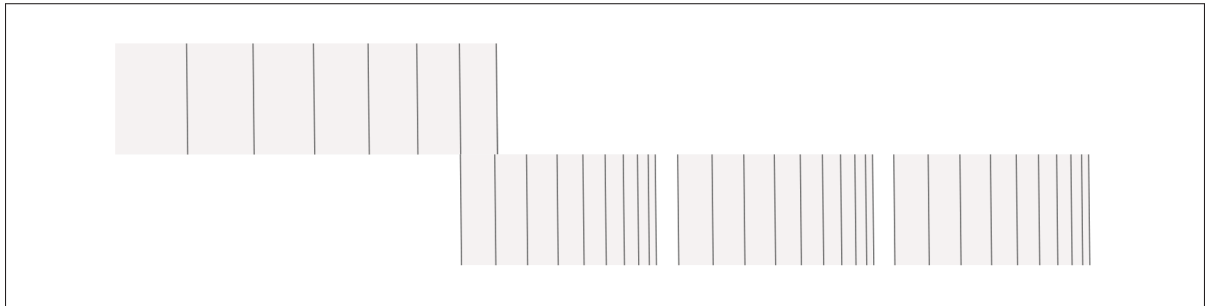
Figure 2.17 Explicit 6: 145 ms, 75-275 Hz and maximum amplitude. A sequence of vibration from one device to the other to evaluate different patterns
