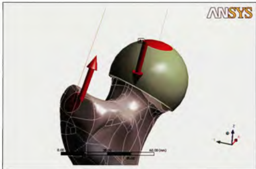
Figure 3.15 Application des chargements.
