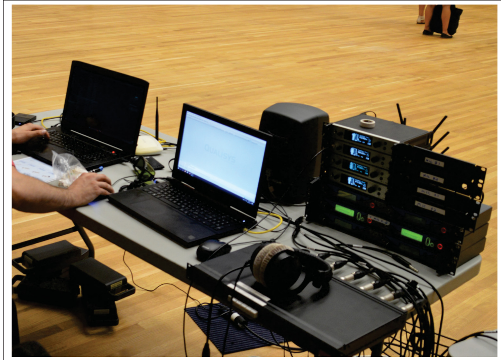
Figure 2.5 Experimental material: two computers, three stereo transmitters, and six mono receivers
