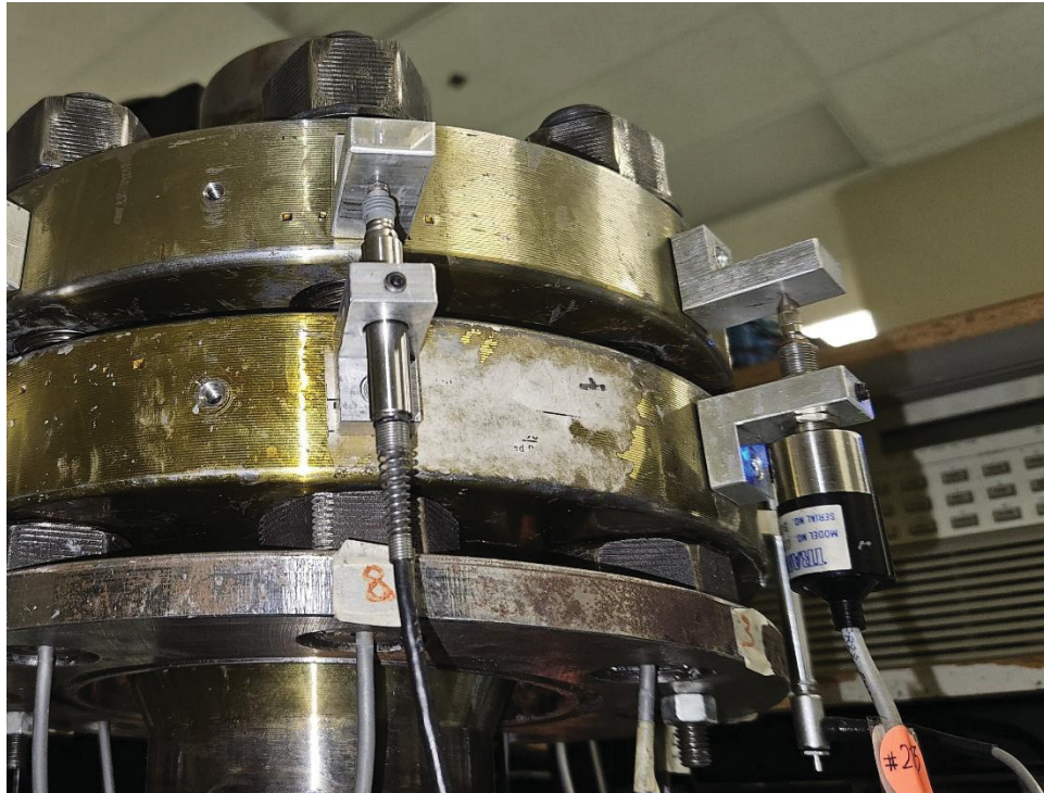
Figure 2.2 LVDTs placed radially on the flange face
