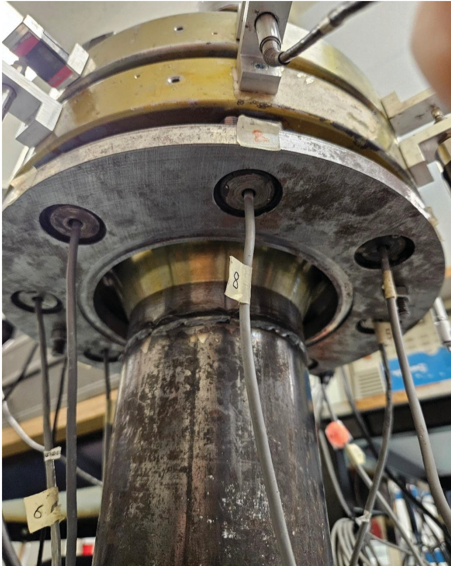
Figure 2.4 strain gauges embedded within the bolts
