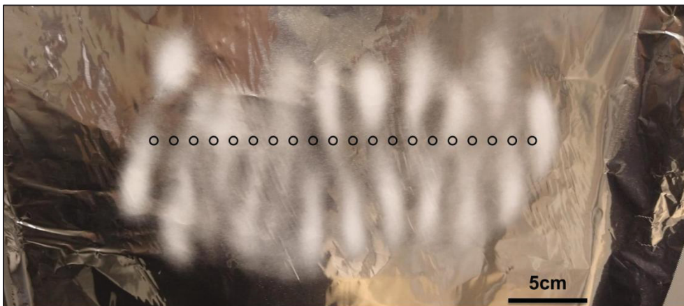
Figure 7.6 Deposition pattern with parallel plate auxiliary electrodes; black circles represent needle position
