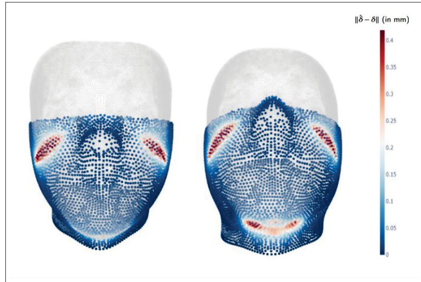
Figure 2.3 Heat map of deformation errors per point (mm) under a mask tightening of 11 N. The colors encode the absolute Euclidean error \|\hat{\delta} - \delta\| (in mm). The largest deviations are concentrated in areas of high curvature (chin); the color bar is indicated in mm
