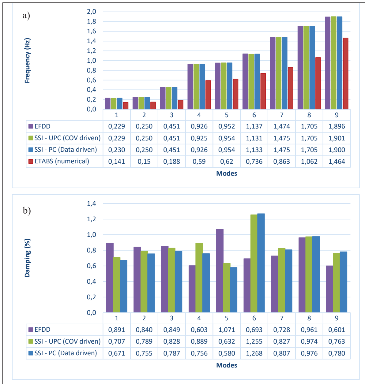
Figure 3.8 Comparison of in-situ and initial numerical modal analysis results a) frequencies and, b) damping ratios
