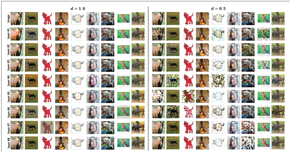
Figure-A I-1 The effect of the token-level stylization on different layers of the Vision Transformer model (encoder). The left and right figures show the results of the reconstructed images when all and half of the tokens are stylized, respectively
