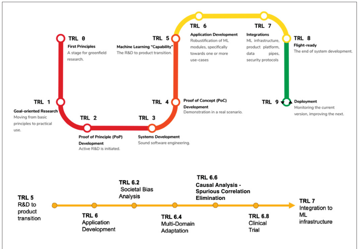
Figure 0.2 Technology Readiness Levels of ML Systems. Medical CV applications often skip levels TRL5 and TRL6 where algorithms are made robust and production ready. Image sources: Lavin et al. (2022) (top); Vlontzos et al. (2022) (bottom)
