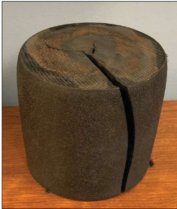
Figure 1.4 Quench test specimen made of 300M steel (treated multiple times) Reproduced with the authorization of SAFRAN
