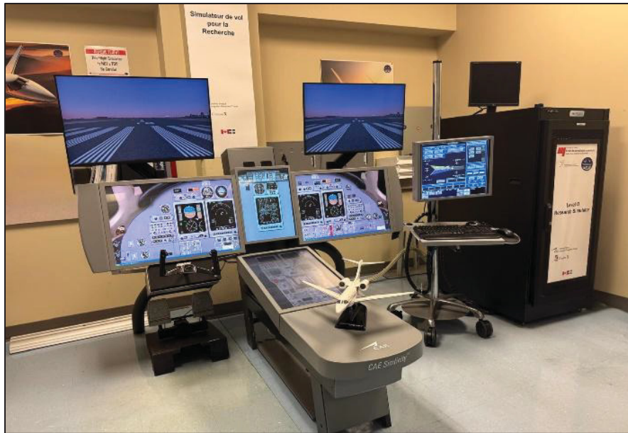
Figure 4.1 Research Aircraft Flight Simulator of the Cessna Citation X available at LARCASE laboratory
