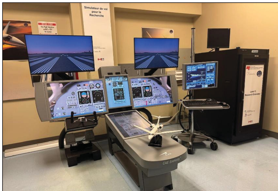
Figure 2.1 Cessna Citation X Research Aircraft Flight Simulator (RAFS) manufactured by CAE
