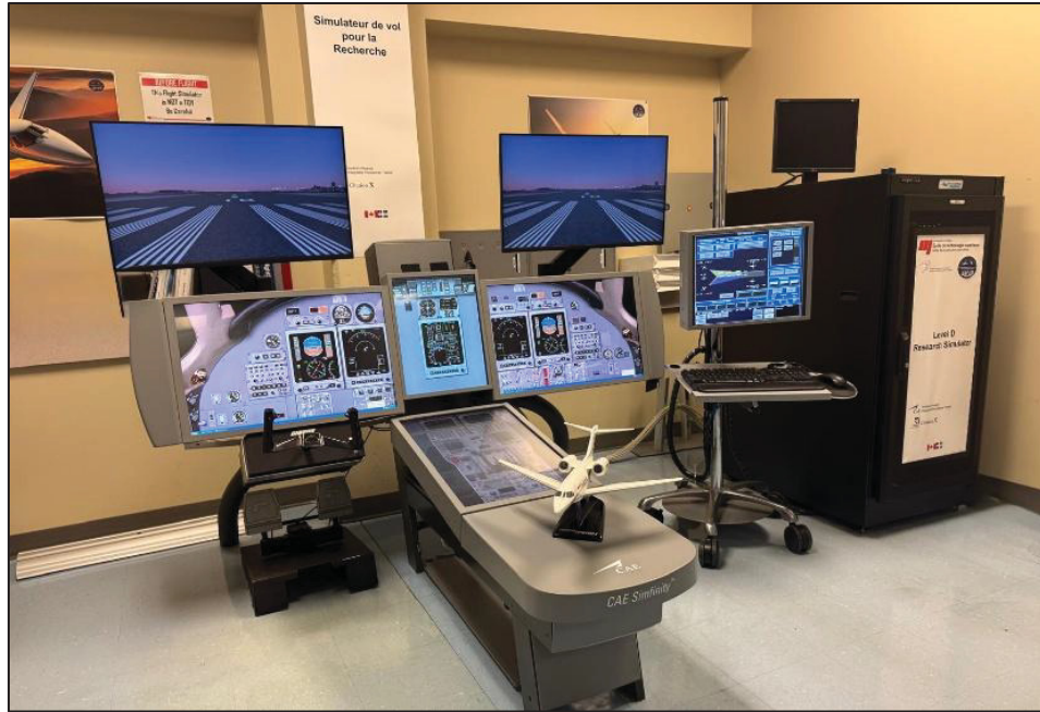
Figure 3.1 Cessna Citation X Level D Research Aircraft Flight Simulator (RAFS) manufactured by CAE.Inc
