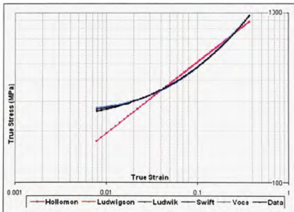
**Figure 3.18** True stress-strain curve of SS 321 tubes 0.9 mm thick fitted by calculated hardening equations in the logarithmic scale.
