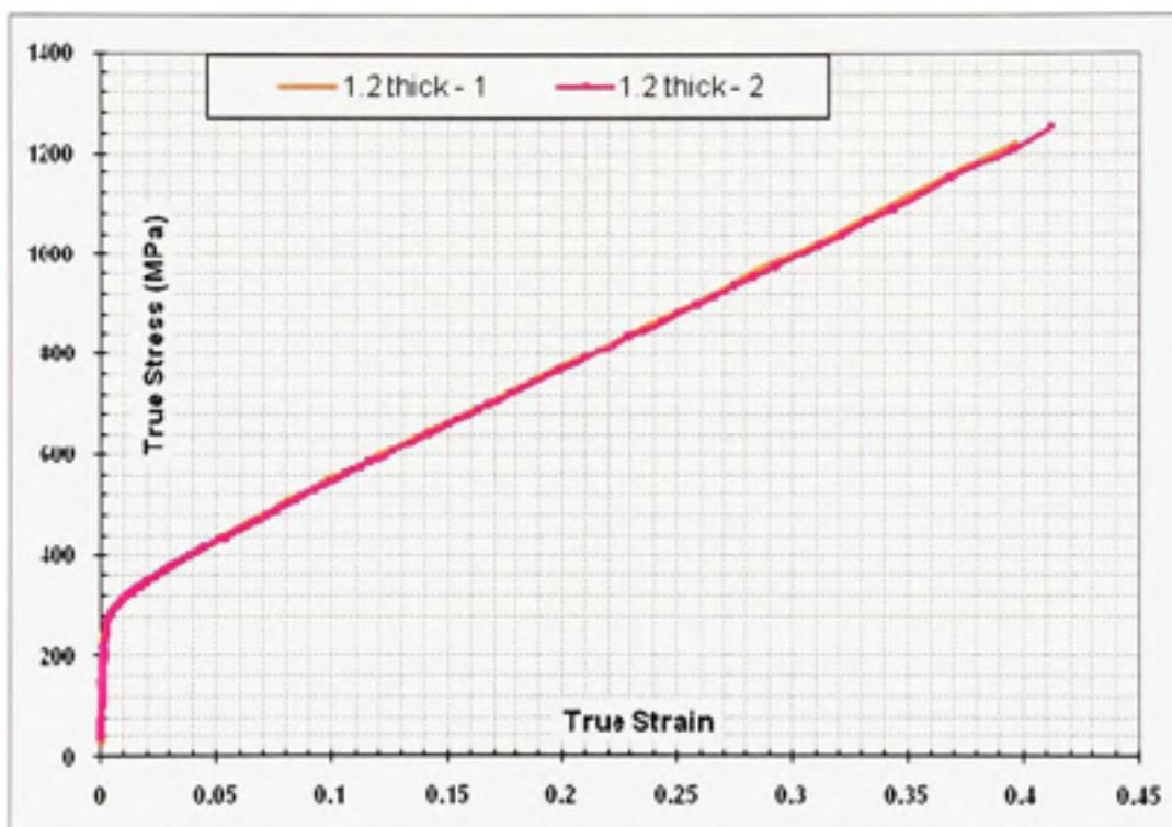
Figure-A-V.1 Engineering stress-strain curves of SS 321 tube samples cut all over the tube – 1.2 mm thick.
