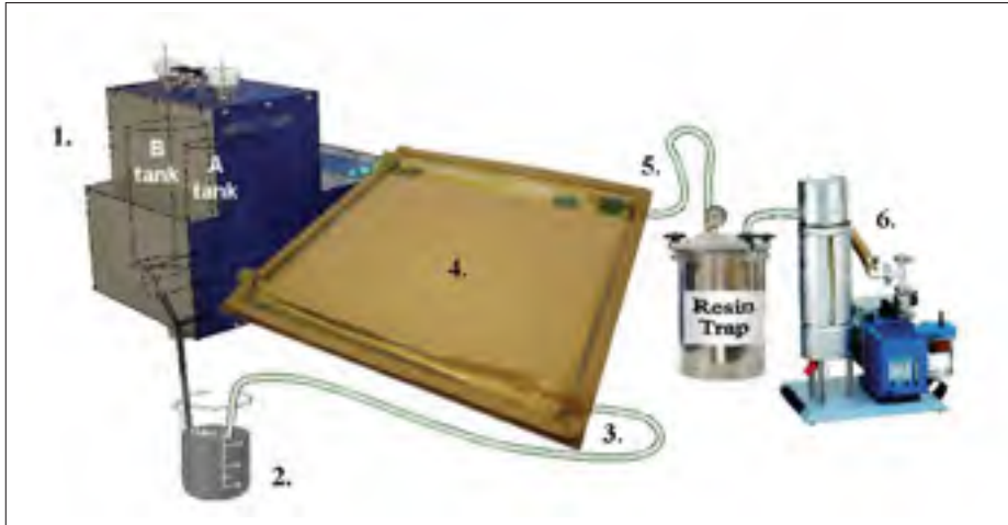
Figure 2.1 Process schematics: (1.) Mini Mixing Unit “MMU-TU Delft”, (2.) resin buffer vessel, (3.) inlet tube, (4.) mould and heating system, (5.) outlet tube and (6.) pressure control system.
