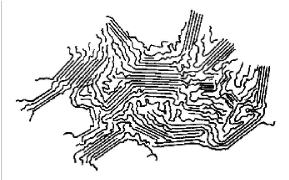
Figure 1.3 Planar zigzag representation of molecules in a semi-crystalline polymer.
