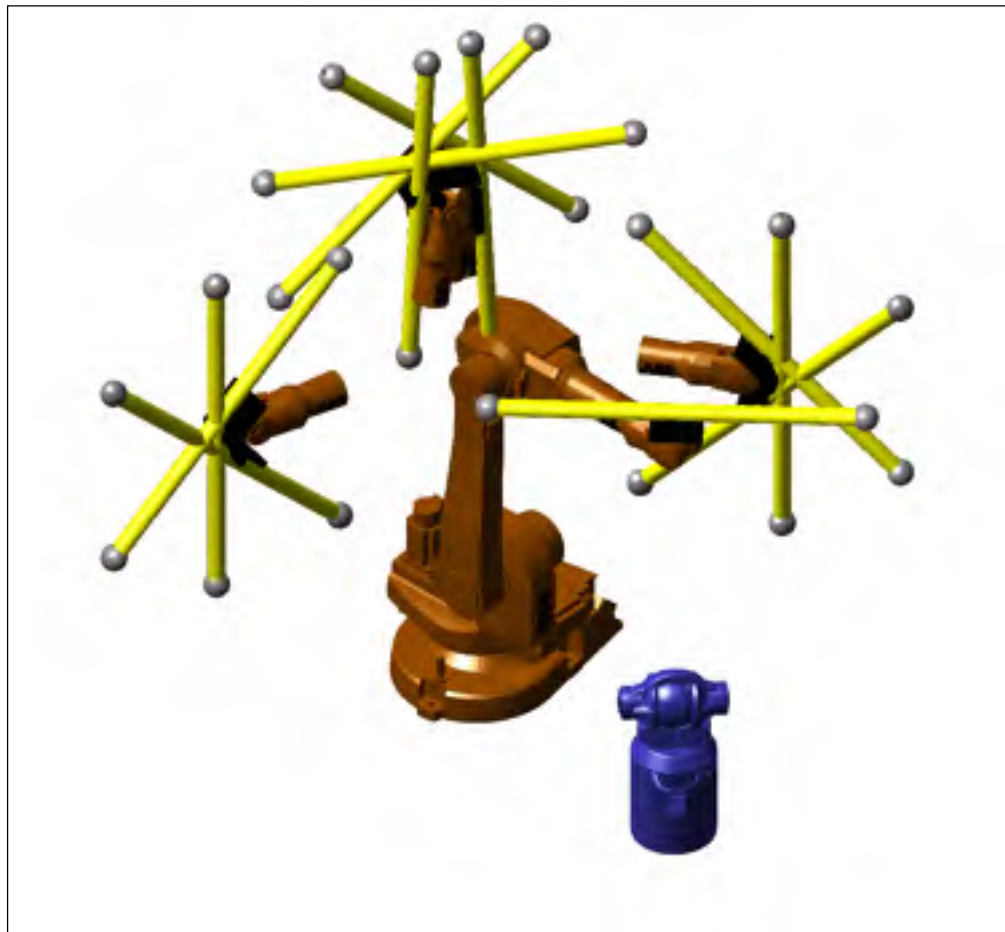
Figure A II-2: Representation of the 12 position tests for measuring the INVAR distance
