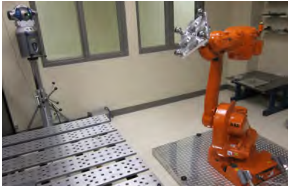
Figure 4.1 The IRB 1600 robot of which the positioning performance was analyzed using a Faro laser tracker
