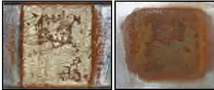
Figure 4.7 Surface deposits on the insulation surface and on the grounded electrode of one PD site
