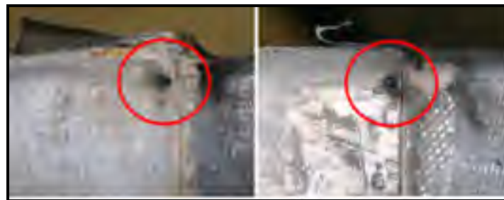
Figure 2.7 Failures sites of one slot PD site of bar 3B (left) and one site of bar 3A (right)
