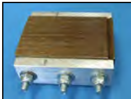
Figure 2.2 Lamination stack used for mechanical abrasion
