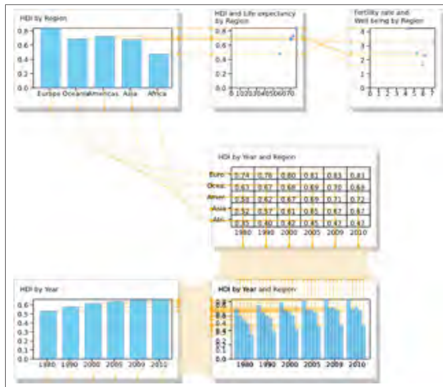
Figure 3.8 Examples of different connections between charts. Top left to top center: tuples are connected across the same Q axis (Mean HDI). Top center to top right: tuples are connected across different Q axes (Mean HDI and Fertility rate). Top left to middle row: values of a C axis (Region) are connected. Middle row to bottom center: an entire C axis is connected to another C axis (Year). Bottom left to bottom center: an entire Q axis is connected to another Q axis (Mean HDI).
