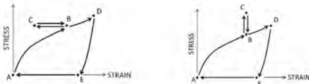
Figure 2. schematization of typical loading paths for a single level of a) constant-stress and b) constant strain
