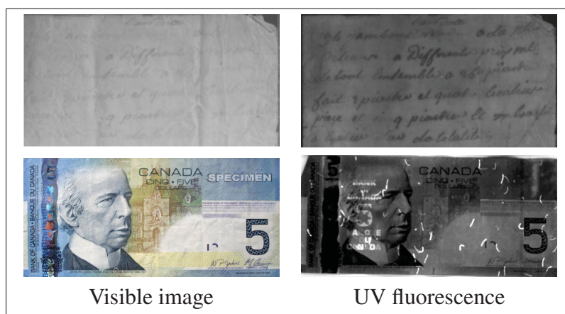
Figure 1.3 The use of UV fluorescence to reveal the faded ink and highlight integrated strips
