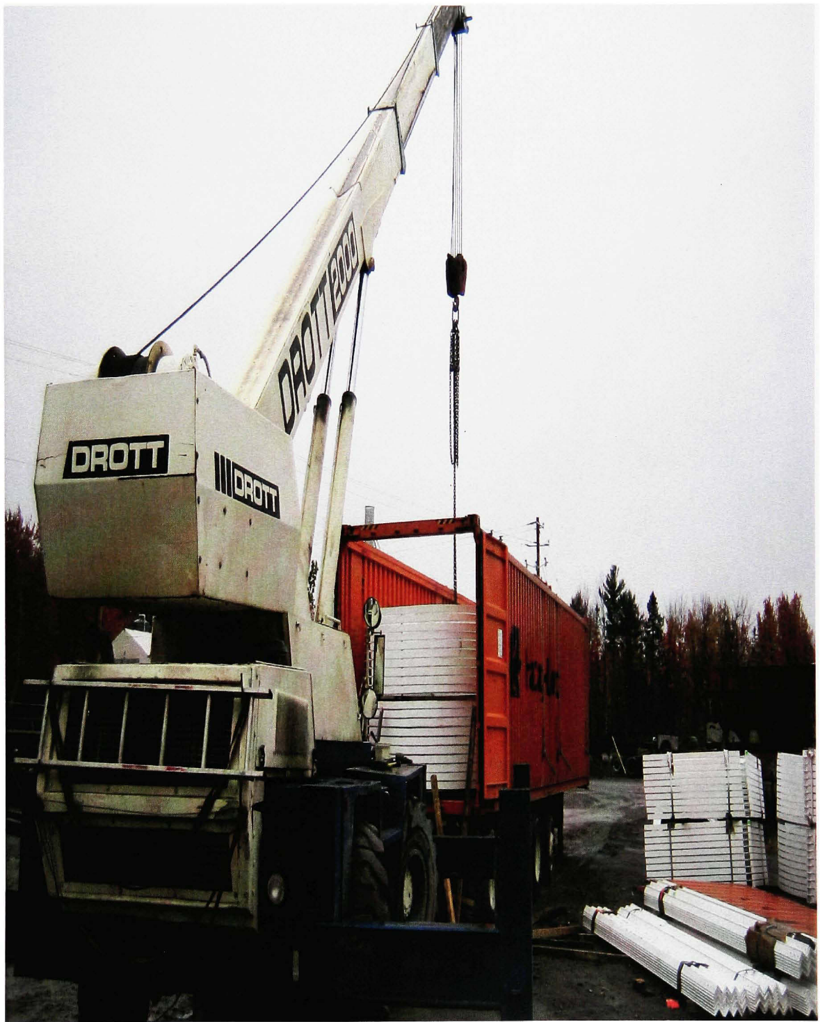
Frame components post fabrication at Air-Therm works scanned and approved being loaded for transport to jobsite
