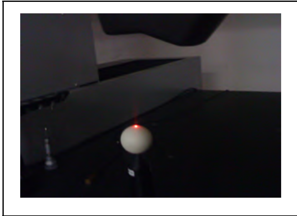
Figure 4.3. Calibration of the laser scanner for the preform scanning
