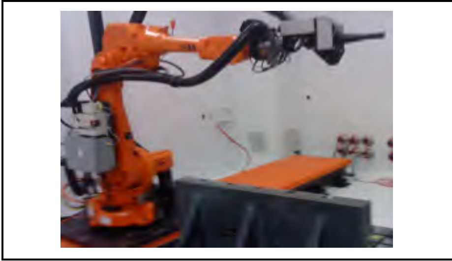
Figure 2.29. Experimental setup for the laser ultrasonic scanning (Courtesy of CTA)
