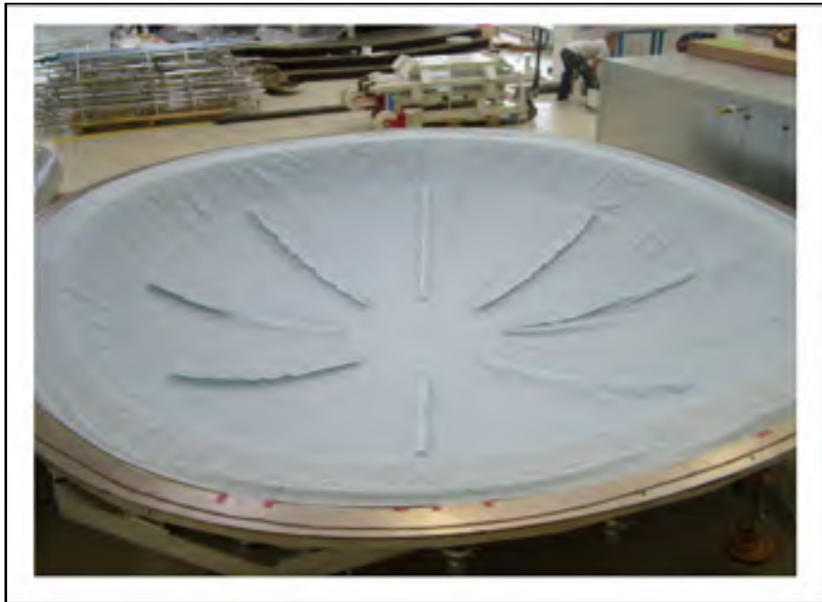
Figure 1.22. Fabrication of pressure bulkhead using vacuum infusion process (courtesy of Trans-Textil GmbH)
