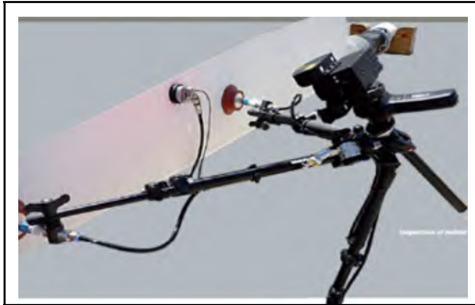
Figure 1.39. The blade inspection using shearography technique (courtesy of Edevis Company)
