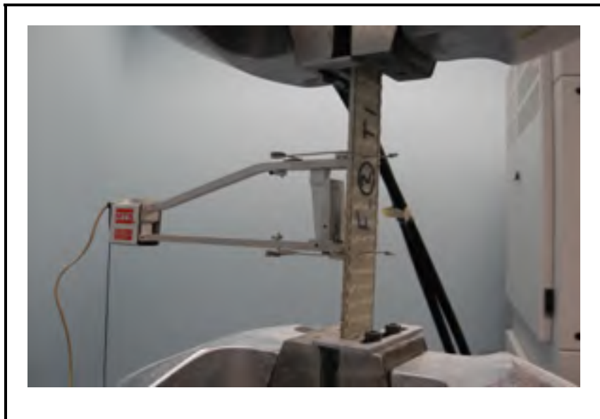
Figure 4.12. Tension test specimen and extensometer for fatigue test.
