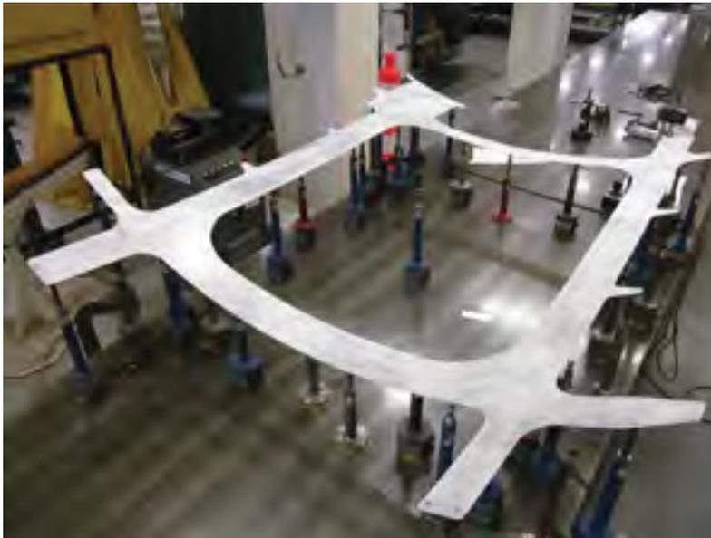
Figure 0.1 Inspection fixture for an aluminum part
