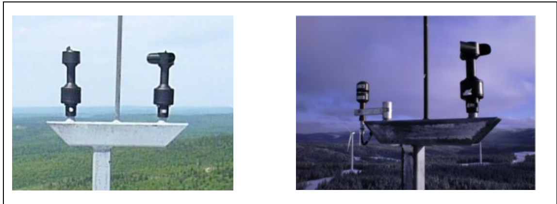
Figure 5-10 Nacelle instrumentation pre- (left) and post- (right) installation of sonic anemometer
