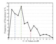
FIGURE 3: Histogram of the C-A values of NIOSH100 noise source database. The C-A of the noise sources used in this study are -1, 2 and 5 dB
