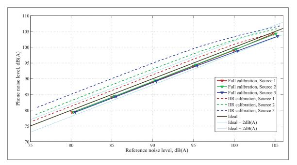
Figure 3.37 Earpiece noise level measurements, while measuring Sources 1,2, 3 in the **reverberant** chamber, with only a frequency-dependent calibration (*FIR calibration*) and with frequency and level-dependent calibration (*Full Calibration*)
