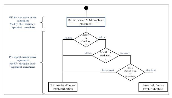
Figure 4.2 User-defined adjustment preliminary flow of questions, associated with the proposed calibration method
