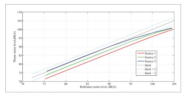
Figure-A VIII-2 Phone noise levels measured with the earpiece, as compared with the reference noise levels while measuring Source 1, 2 and 3 in the semi-anechoic chamber with the phone implementing the frequency-dependent calibration algorithm
