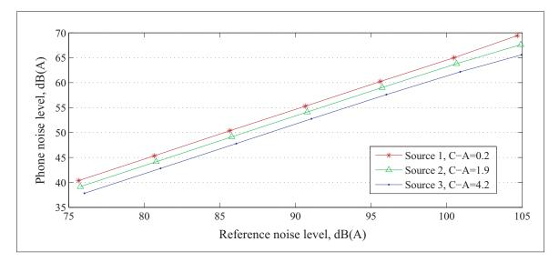
Figure-A VIII-1 Uncalibrated mobile phone noise levels measured with the earpiece, as compared with the reference noise levels while measuring Source 1, 2 and 3 in the semi-anechoic chamber
