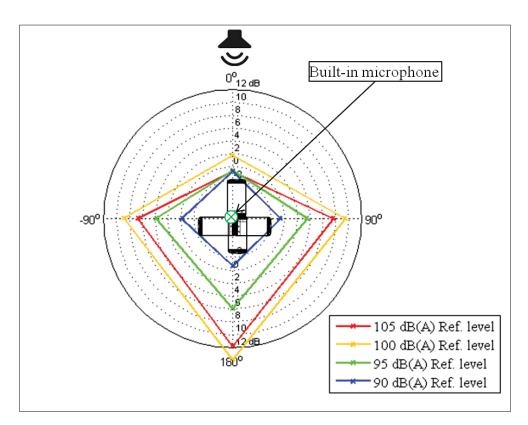
Figure 3.34 Built-in microphone overall A-weighted errors for various microphone placement and noise levels, while measuring Source 1 in the semi-anechoic chamber
