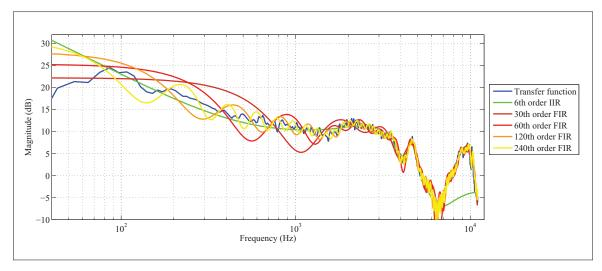
Figure 3.21 Frequency responses of IIR calculated from the truncated-transfer functions and frequency responses of FIR filters for orders from 30<sup>th</sup> to 240<sup>th</sup> order based on the initial built-in microphone transfer function
