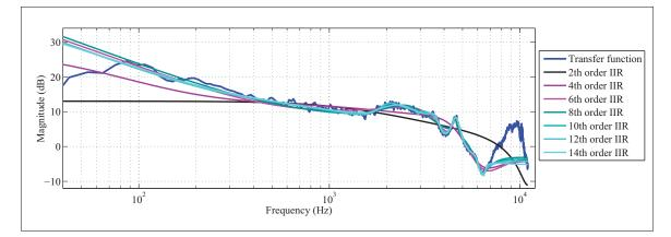
Figure 3.17 Built-in microphone initial transfer function, defined from 0 to 11025 Hz, and frequency responses of IIR filters for orders from 2 to 14, calculated from the truncated-transfer function (from 80 Hz to 6700 Hz)
