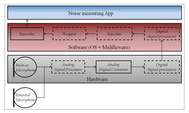
Figure 1.2 Hardware and software components of the audio recording path of mobile phones
