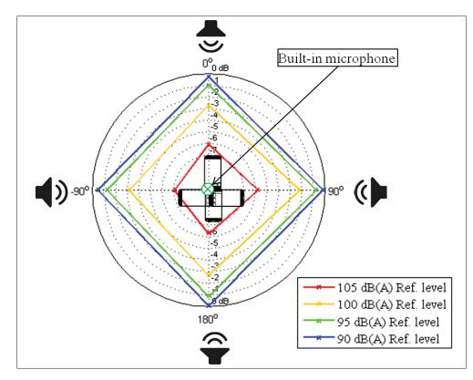
Figure 3.35 Built-in microphone overall A-weighted errors for various microphone placement and noise levels, while measuring Source 1 in the reverberant chamber
