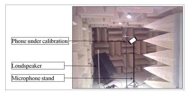
Figure 2.15 Setup of the calibration measurement in the semi-anechoic chamber showing a mobile phone under calibration and the loudspeaker
