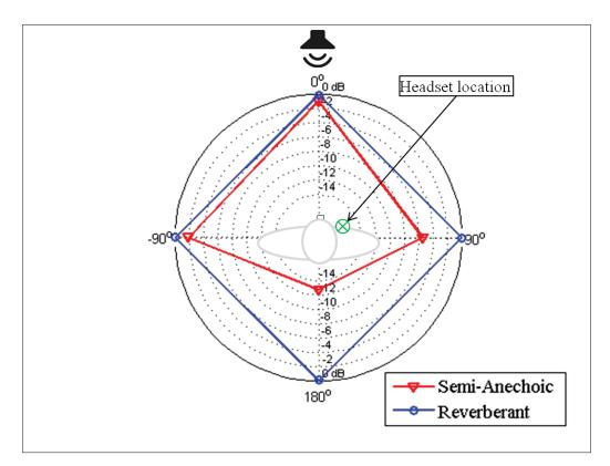
Figure 3.31 Headset overall A-weighted errors, averaged over the range of noise levels, in the semi-anechoic chamber (in red) and in the reverberant chamber (in blue)
