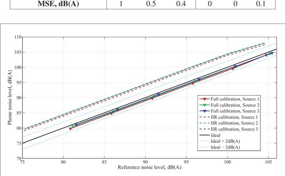
Figure 3.29 Headset noise level measurements carried out in the **semi-anechoic** chamber, with only a frequency-dependent calibration (IIR calibration) and with frequency and level-dependent calibration (Full Calibration)
