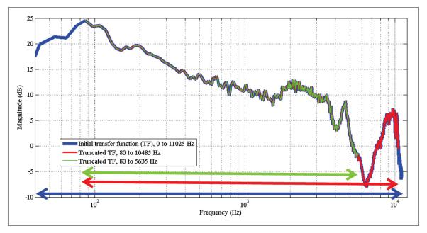
Figure 3.15 Initial transfer function (in blue) based on the built-in microphone measurement, truncated-transfer functions, defined from 80 Hz to 10485 Hz (in red) and to 5635 Hz (in green)
