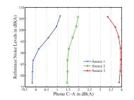
FIGURE 7: Reference noise levels in dB(A) as a function of phone C-A in dB(A)
