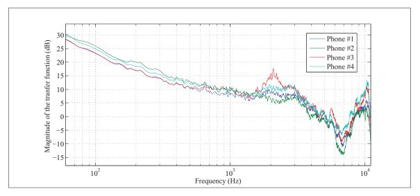
Figure 3.10 Transfer functions calculated from the built-in microphone measurements of the 4 ZTE N762 mobile phone units
