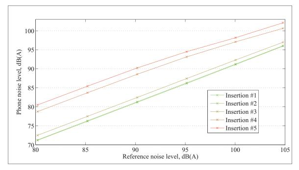
Figure 3.14 Noise level corrections measurements for five variations of earpiece placement within the built-in ear simulator measured in the semi-anechoic chamber
