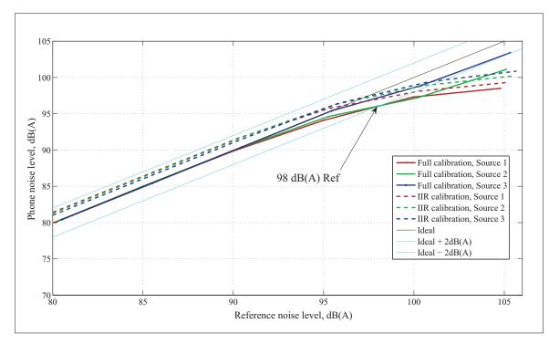
Figure 3.33 Built-in microphone noise level measurements in the **reverberant** chamber with only a frequency-dependent calibration (FIR calibration) and with frequency and level-dependent calibration (Full Calibration)
