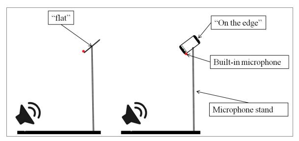
Figure 2.22 Side view of the built-in microphone orientation in the semi-anechoic chamber: mobile phone placed flat (on the left) and on the edge (on the right)
