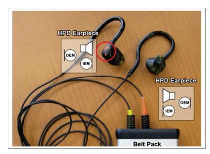
Figure 2.10 Sonomax<sup>®</sup> earpiece from the individual dosimetric hearing protection with the emplacement of the microphone encircled in red adapted with the permission from Mazur and Voix (2013)
