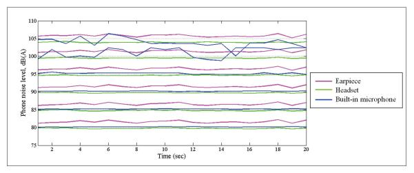
Figure 3.28 Built-in microphone, headset and earpiece  $L_{eq,A,1sec}$ , measured during the validation measurements for 6 noise levels
