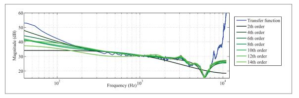
Figure 3.20 Earpiece initial transfer function for the earpiece located on a stand and frequency responses of IIR filters for orders from 2 to 14
