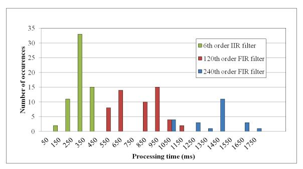
Figure 3.23 Histogram of the processing time required by the mobile phone app to compute a  $L_{eq,A,1sec}$  over a one-minute-measurement and depending on the IIR and FIR filters order
