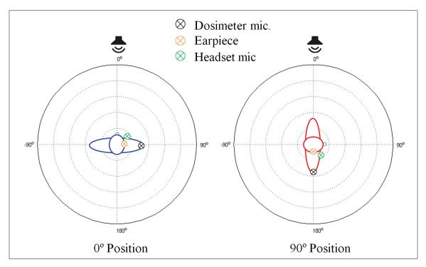
Figure 2.18 Top view of 2 of the 4 ATF positions relative to the source in the semi-anechoic chamber
