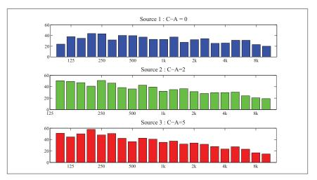
Figure 2.3 Noise spectrum of Sources 1, 2 and 3 with C-A value of 0, 2 and 5 respectively
