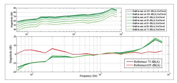
Figure 3.4 Frequency responses of the measurements conducted with the built-in microphone (top half), frequency responses with the magnitude normalized at the 1 kHz third-octave band noise level (top bottom)
