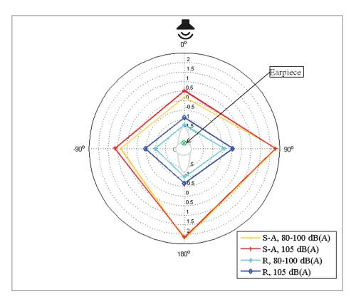
Figure 3.40 Earpiece overall A-weighted errors in the semi-anechoic chamber (in red an orange) and in the reverberant chamber (in blue)
