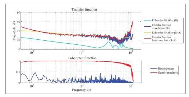
Figure 3.22 Earpiece transfer function and coherence values, frequency responses of 12<sup>th</sup> order IIR filters
