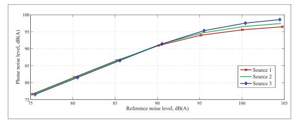
Figure 3.24 Built-in microphone noise level with a frequency-dependent calibration (6th order IIR filter), function of the reference noise level, while measuring Source 1, 2, 3
