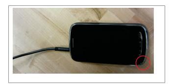
Figure 2.9 Unit of ZTE N762 mobile phone with the adapter cable plugged into the phone' audio input and the built-in microphone encircled in red
