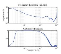
$\label{eq:Figure 4: Frequency response function and coherence between a smartphone and the reference measurement system with dual channel FFT analysis$
