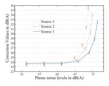
$\label{eq:FIGURE 6: Correction values in dB(A) as a function of the phone noise levels and their associated expanded uncertainties in error bars$
