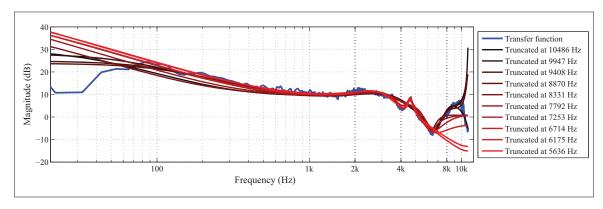
Figure 3.16 Initial transfer function based on the built-in microphone measurement and frequency responses of 6th-order IIR filters calculated from the truncated-transfer function, defined from 80 Hz to several truncated-end starting at 10485 Hz until 5635 Hz
