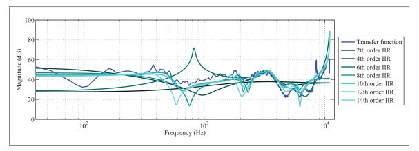
Figure 3.19 Earpiece initial transfer function for the earpiece located on the ATF and frequency responses of IIR filters for orders from 2 to 14
