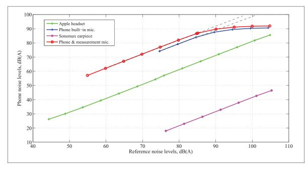
Figure 3.2 Mobile phone noise levels measured in the anechoic chamber while measuring Source 1
