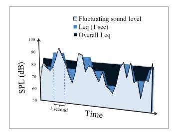
Figure-A II-1 Fluctuating sound pressure level, Overall  $L_{eq}$  and short  $L_{eq}s$
