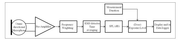
Figure-A III-2 Simplified block diagram of a noise dosimeter
