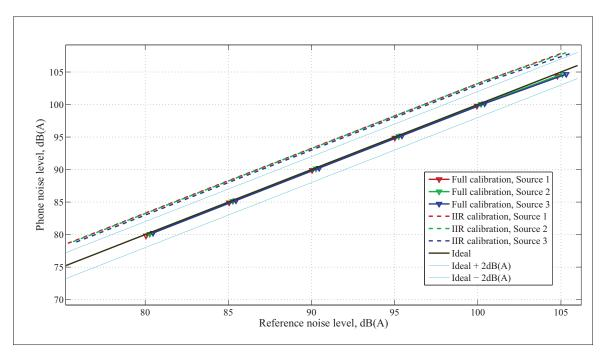
Figure 3.30 Headset noise level measurements carried out in the **reverberant** chamber, with only a frequency-dependent calibration (IIR calibration) and with frequency and level-dependent calibration (Full Calibration)
