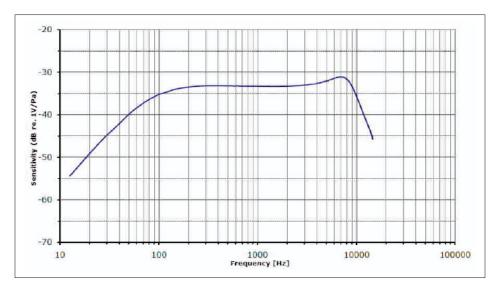
Figure 2.12 Frequency response of the Sonomax<sup>®</sup> earpiece microphone, extracted from Sonion (2009)
