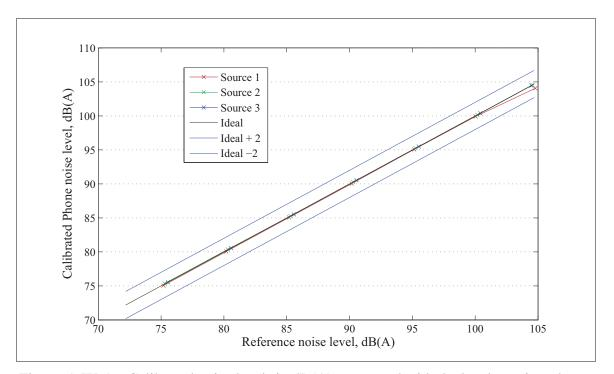
Figure-A IX-1 Calibrated noise levels in dB(A), measured with the headset microphone, right after the calibration measurement
