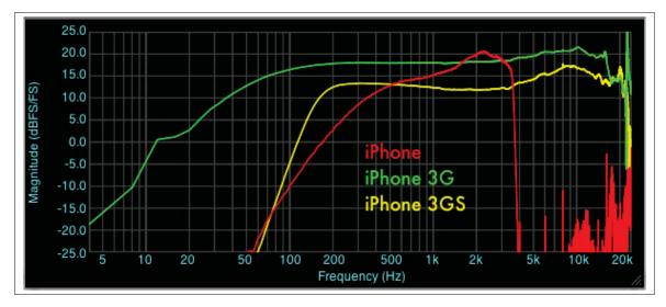
Figure 1.7 Built-in iPhone Microphone Frequency Response Comparison. Reproduced with the permission from Faberacoustical (2009)
