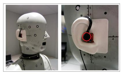
Figure 2.13 Sonomax<sup>®</sup> earpiece on the ATF's built-in ear simulator with the location of microphone encircled in red
