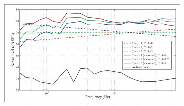
Figure 2.5 Frequency content of the ambient noise, the original signals of Sources 1, 2 and 3 and the measured Sources 1, 2 and 3 with the reference system in the semi-anechoic chamber
