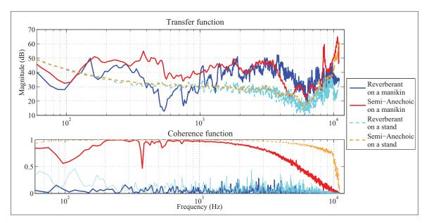
Figure 3.11 Transfer function and coherence values calculated from earpiece measurements in the semi-anechoic and reverberant chambers with the earpiece on a stand and on the ATF
