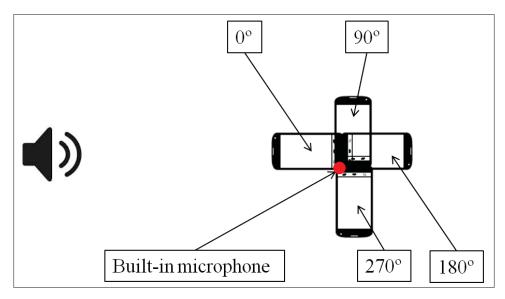
Figure 2.21 Top view of the built-in microphone orientation in the semi-anechoic chamber with the mobile phone placed flat
