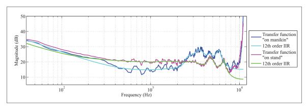
Figure 3.18 Headset transfer functions based on the measurement for different microphone placements and frequency responses of the 12<sup>th</sup> order IIR filters, calculated from the truncated-transfer functions (from 43 Hz to 7250 Hz)
