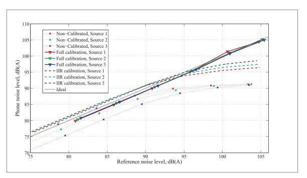
Figure 3.32 Built-in microphone noise level measurements in the **semi-anechoic** chamber without calibration, with only a frequency-dependent calibration (IIR calibration) and with frequency and level-dependent calibration (Full Calibration)
