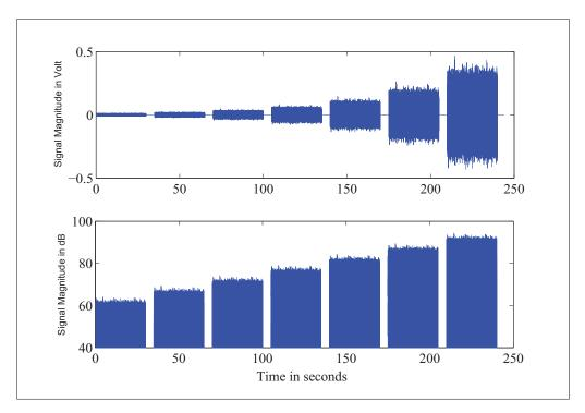
Figure 2.4 Sequence of 7 30-seconds signals of Source 1 with the noise level increasing by 5 dB every time and with a 5 second silence between each signal
