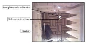
$\label{eq:FIGURE 1: Setup of the calibration measurement in the anechoic chamber showing the smartphone under calibration, the reference microphone and the powered speaker$
