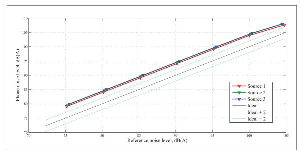
Figure-A VIII-4 Phone noise levels measured with the headset, as compared with the reference noise levels while measuring Source 1, 2 and 3 in the semi-anechoic chamber with the phone implementing the frequency-dependent calibration algorithm
