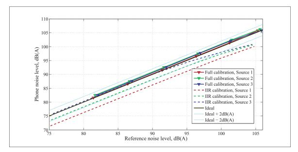
Figure 3.36 Earpiece overall A-weighted errors measured in the **semi-anechoic chamber** with only a frequency-dependent calibration (*FIR calibration*) and with frequency and level-dependent calibration (*Full Calibration*)
