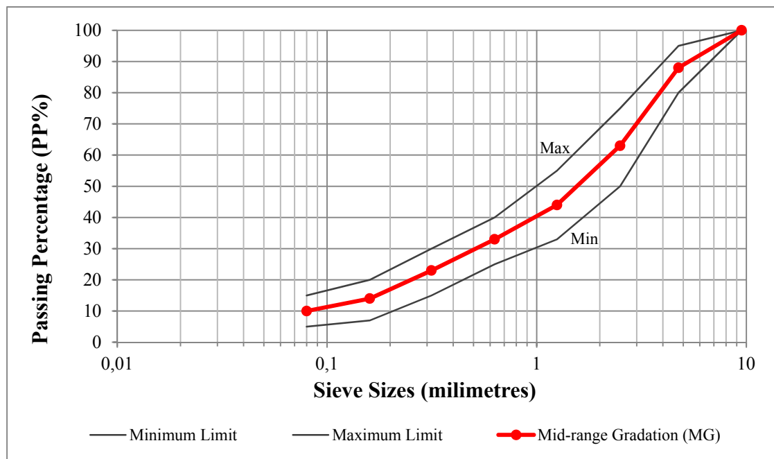
Figure 8.1 Middle aggregate gradation curves (Ray-Car 0-5 mm size)
