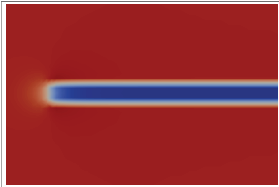
Figure 2.10 Lightly loaded actuator disk case: wake development.
