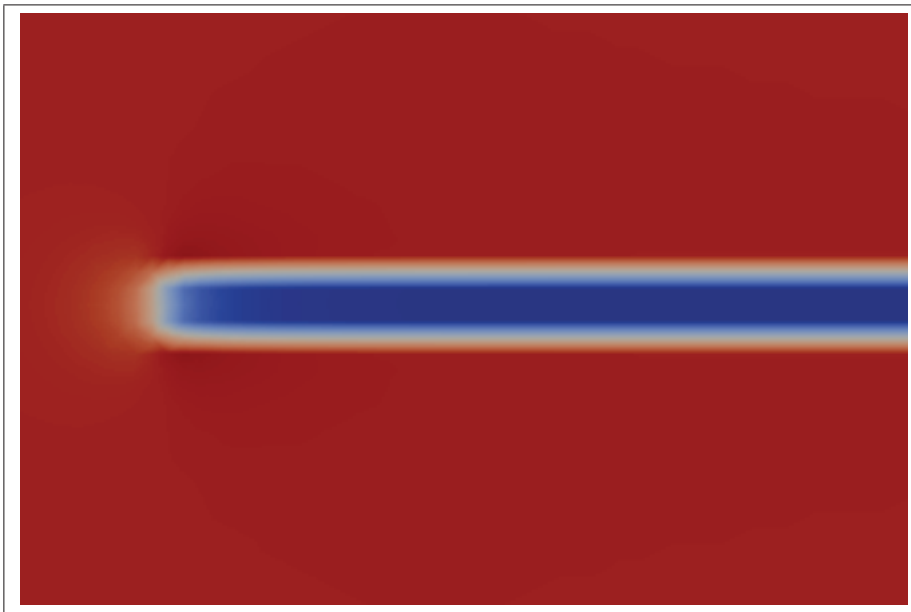
Figure 2.10 Lightly loaded actuator disk case: wake development.
