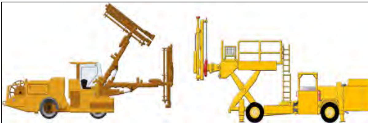
Figure 5.1 Semi-automated bolter VS standard bolter
